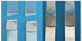
**Homopolymer PP** SG400LSE's tough bond results in substrate failure
